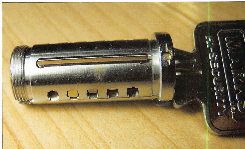
Photo 7, The bottom of the plug with the finger pins at the various depths.
