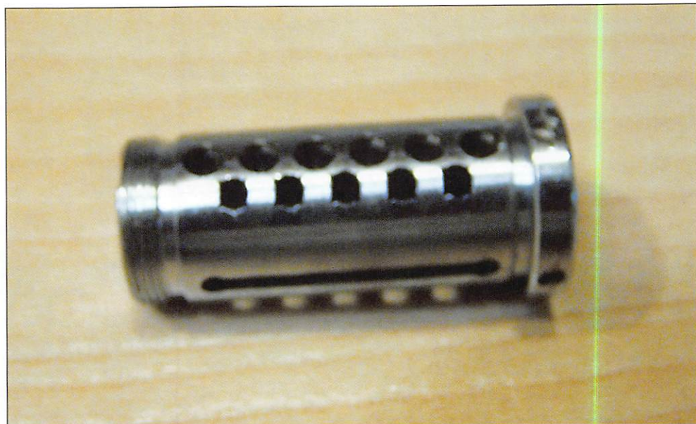
Photo 6, The second set of holes for the finger pins are next to the pin chamber holes.
