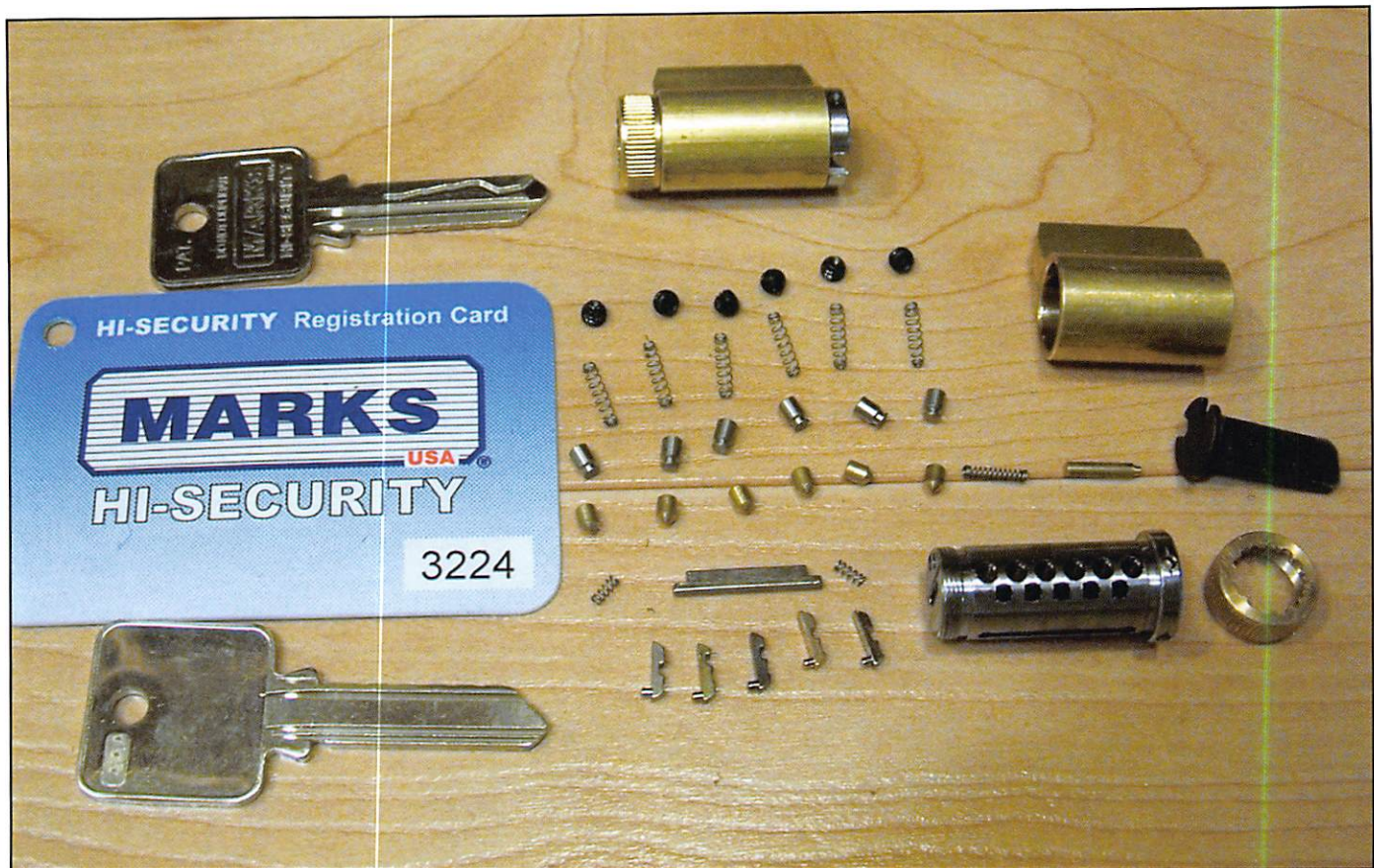
Photo 1, The non-UL cylinder is disassembled. Above it is the UL listed version. Also shown in the picture is the signature card for additional keys.
